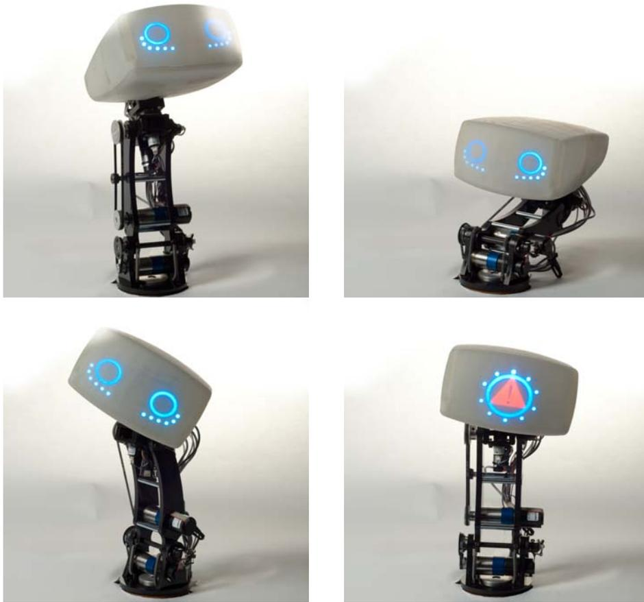
Figure 3.2: The current AIDA implementation with fully functional mechanical systems and embedded projector.
