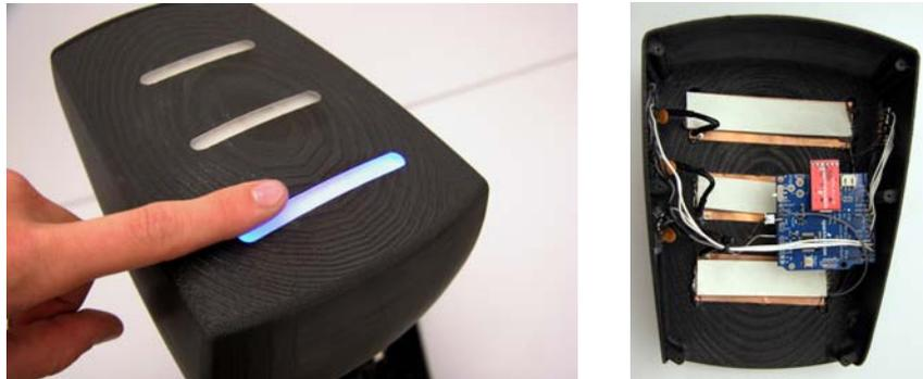
Figure 3.4: Figures showing an AIDA head shell responding to integrated capacitive touch sensing (left) and the internal electronics (right).
